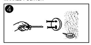
4.TIGHTEN THE STAINLESS STEEL SCREWS WITH A SCREWDRIVER AND FIX THE GASKET
