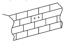
Refer to product size, drill 6mm holes on the appropriate position of wall surface.
