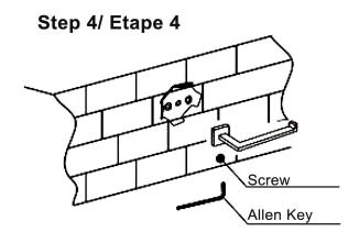
Finally,hang the main body to thrust on thewall, tighten screws with spanner,confirm installment is reliable
