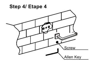
Finally,hang the main body to thrust on thewall, tighten screws with spanner,confirm installment is reliable
