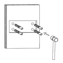
4). Use a Phillips screwdriver to tighten the 4 self-tapping screws, fix the valve body on the wall.
