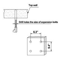
4). Insert the shower fixed seat into the four expansion bolts to adjust the nuts to fit the ceiling is on the same plane, and finally Finally, the square hole ceiling is buckling up to the suspended ceiling board.
