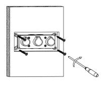
5). Draw a line while aligning the installed embedded box, and figure the installation distance, Dimension as below is for reference, which should be adjusted in reality. Then drill on wall for water pipe in final.
