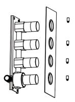
3). With reference to the basic dimensions of the embedded body, excavate the embedded ports of the main body, hot & cold water inlet pipe and the outlet pipe.
