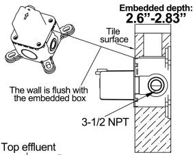
2. After the main body is buried in the wall, remove the lid of the Embedded Box; place the trim plate and mount the handles.
