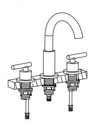
4. Connect the pipe of spout and two handles.
