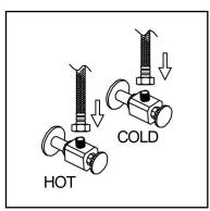
5. Attach flexible hose to water supply.
