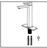
2. Screw and hand tighten the hot and cold flexible hoses to the faucet. DO not use a wrench to tighten hoses as this may damage the hose and/or the hose threads.
