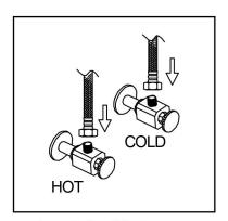
5. Attach flexible hose to water supply.
