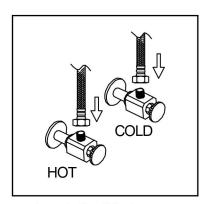
5. Attach flexible hose to water supply.
