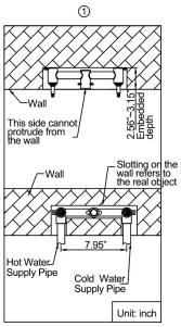
1. Make a groove in the wall as shown, the depth must be be consistent with the valve body, refer to the real item. Connect the pipes when embedding the valve, and check if there is any leakage.
