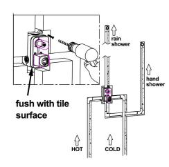
3. Fix ceramic tiles, cut off the edges of the embedded box, remove the protective cover and install the panel.
