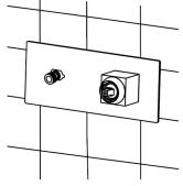
7. Mount the outlet pipe by tighten two screw with wrench.
