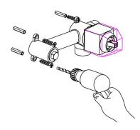
3. Remove Protect cover and plug after Installing of Body.
