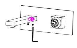
8. Mount the handle by tighten two screw with wrench, and then cover decoration button.
