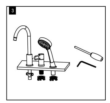
3. As shown in the picture, first install the main body into the bottom, then lock it with the locking assembly, then install each handle on each main body, and finally lock it with a tool.
