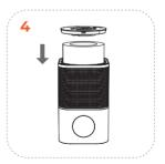
Place the filter into the air purifier and install the base cover properly. Tighten the filter buckle until it clicks into place.
