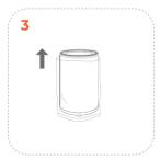
Remove the filter protective bag before installation.
