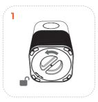
Rotate the twist handle clockwise to unlock the base cover.
