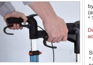
Push the brake handles downwards until they lock into place with "click" to park the rollator. Pull the brake handles back up to release parking position.
