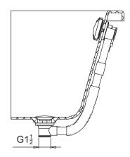
7. Installation of drain pipes:Install the drain pipes to the bathtub according to the installation instructions of the drain pipes .The figure below is the installation illustration recommended by our company for the Drain Pipe P9098N series.
