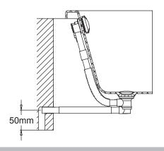
Installation of the drainers:Install the drainers to the bathtub according to the installation instructions of the drainers. The figure below is the installation illustration recommended by our company specificly for the Drainer D409 series.
