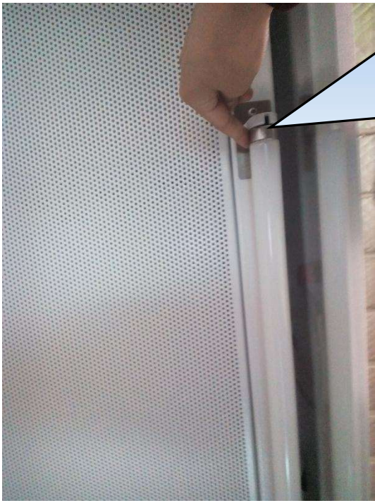
Figure 12 UV lamp replacement diagram
