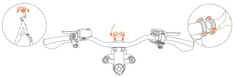
③Adjust the handlebar to the right position, should be in a parallel with the fork; close the handlebar clamp and tighten the screw.
