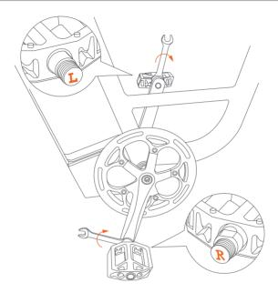
Use the open spanner of the tools bag, screw the pedal shaft into the threaded hole and tighten it in the direction of the arrow.
