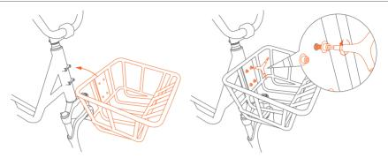
Align the four holes of the front basket with the four holes of the bike head, and tighten screws
