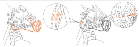
Align the headlights with the front basket hole, put into screws and nuts then tighten, and then insert the the red line and blue line of the headlights in accordance with the direction of the arrow
