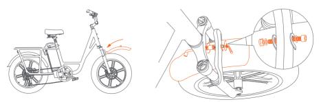
Put the front fender through the gap of the tire and fork, then screw tightenly.
