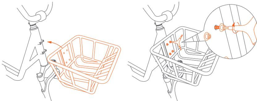
Align the four holes of the front basket with the four holes of the bike head, and tighten screws
