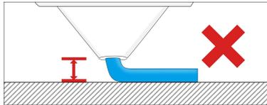
If the distance between the nozzle and the platform is too high, the filament will not easy to stick to the platform. Should click "Decrease" until the distance is proper.
