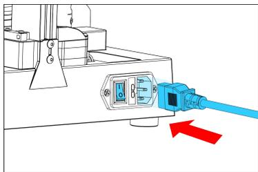
Plug in the cable and turn on the power
