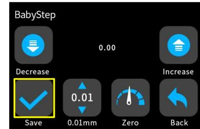
When you start your first printing, adjust the Babystep value according to the adhesion of the filament and the glass platform. Click "Save" to save your setting, and you don't need to adjust the value again next time. **[Note: Z-off set use for the first layer only]**
