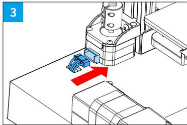
Z Motor 2 cable | Z-Motor 2 Kabel
