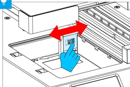
**Note:** The power supply has been adjusted according to the local voltage. If you need to adjust the voltage, please follow the picture to operate it.
