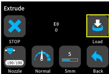
Click "load" to feed the filament until the filament is out of nozzle.
