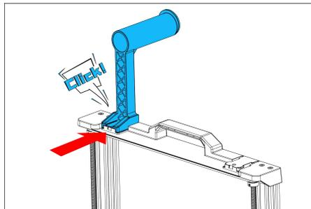
The filament holder can be installed left and right
