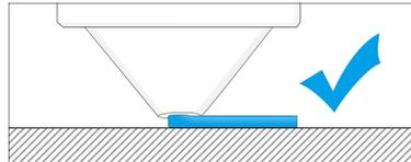
Keep the distance between the nozzle and the hot bed at 0.1mm, the filament will stick to the hot bed evenly
