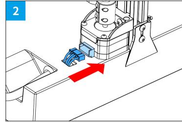
Z Motor 1 cable | Z-Motor 1 Kabel
