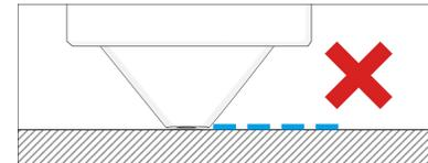
If the distance between the nozzle and the platform is too low, the filament will be not easy to feed out smoothly . Should click "Increase" until the distance is proper.
