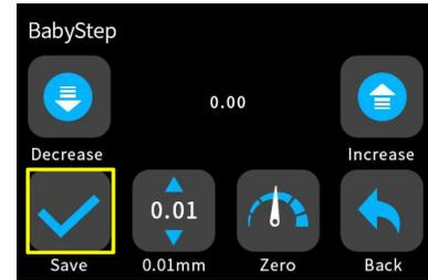
When you start your first printing, adjust the Babystep value according to the adhesion of the filament and the glass platform. Click "Save" to save your setting, and you don't need to adjust the value again next time.
