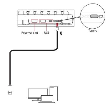
Recommend: Using 5V 1A Rated power to charge keyboard
