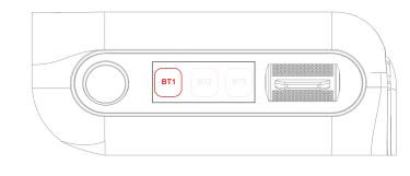
1.Use the toggle to select BT1/BT2/BT3 icon,and connect any group of bluetooth devices. Pairing setting: for example,select BT1,then press and hold "OK"until it shows BT1 is paring, which means that the pairing is in progress.
