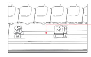
This feature allows you to completely power off the device and then initiate a fresh restart when needed. Simply hold the button located below the space key and on the left side of the switch for 3 seconds to activate this function.
