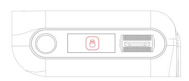
2.4G mode: use the toggle to select the 2.4G icon, and click the push button. Keyboard is switched to 2.4G mode and the display shows "2.4G linking".
