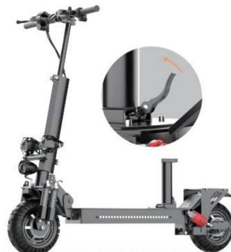
5. Install the seat bag and fix the folding buckle
