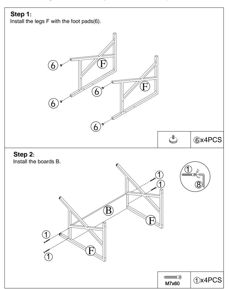
Note: Do not tighten the screws untill you finish all assemble steps.
