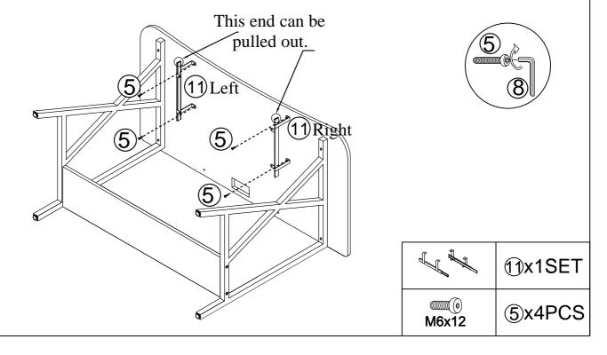
Note: Do not tighten the screws untill you finish all assemble steps.
