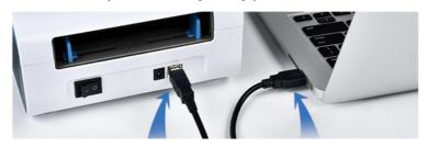
3. Make sure the power adapter is tightly connected, then connect the power cable to the printer's power port and the electrical socket.
