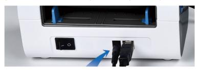
4. Turn the power ON, (Pressing down "—" means turn ON) and you will see the top button shining.
