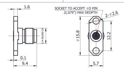
For glass-bead of 0.51mm pin diameter
