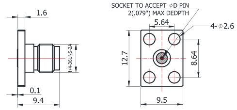
For glass-bead of 0.51mm pin diameter
