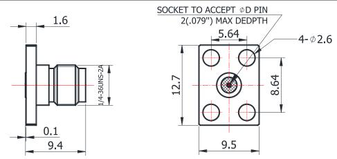
For glass-bead of 0.46mm pin diameter
