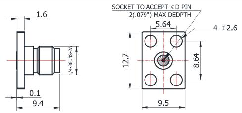
For glass-bead of 0.38mm pin diameter
