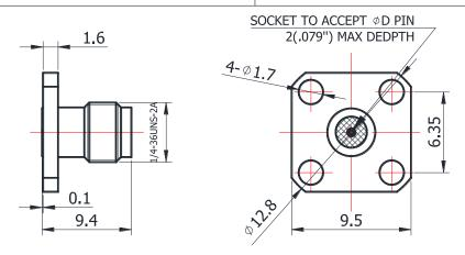
For glass-bead of 0.30mm pin diameter
