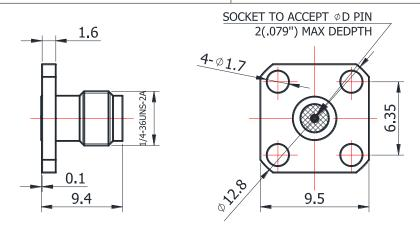
For glass-bead of 0.23mm pin diameter
