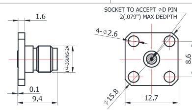
For glass-bead of 0.46mm pin diameter
