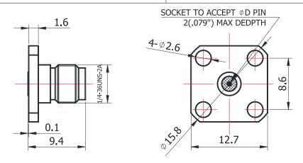
For glass-bead of 0.38mm pin diameter
