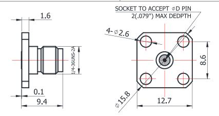
For glass-bead of 0.23mm pin diameter
