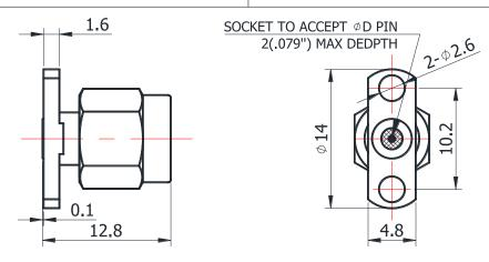
For glass-bead of 0.51mm pin diameter
