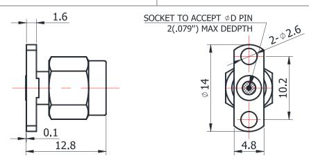
For glass-bead of 0.38mm pin diameter
