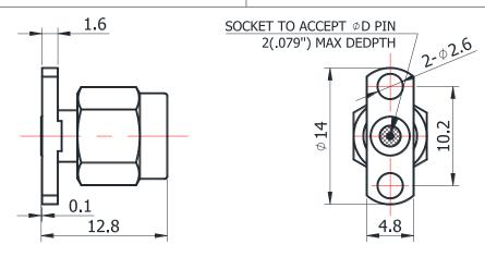
For glass-bead of 0.30mm pin diameter
