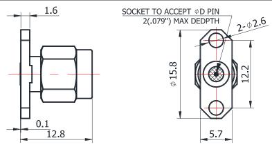
For glass-bead of 0.46mm pin diameter
