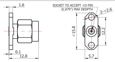
For glass-bead of 0.38mm pin diameter
