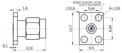
For glass-bead of 0.46mm pin diameter
