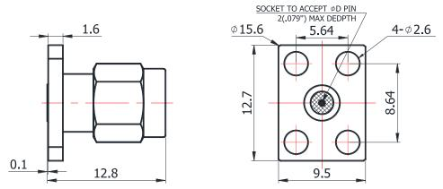
For glass-bead of 0.38mm pin diameter
