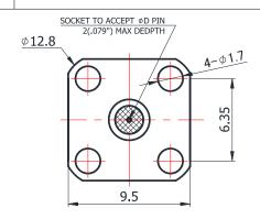
For glass-bead of 0.51mm pin diameter
