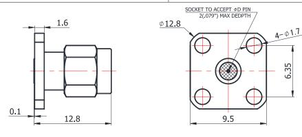
For glass-bead of 0.46mm pin diameter
