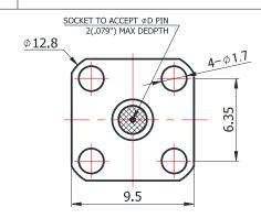
For glass-bead of 0.30mm pin diameter
