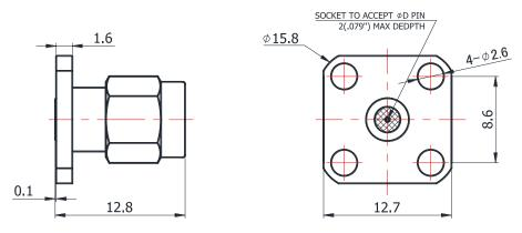
For glass-bead of 0.38mm pin diameter
