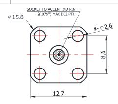
For glass-bead of 0.23mm pin diameter
