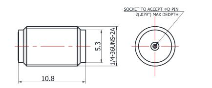
For glass-bead of 0.38mm pin diameter
