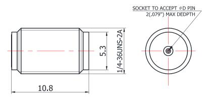
For glass-bead of 0.30mm pin diameter
