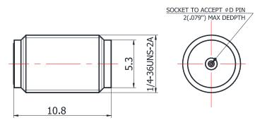
For glass-bead of 0.23mm pin diameter
